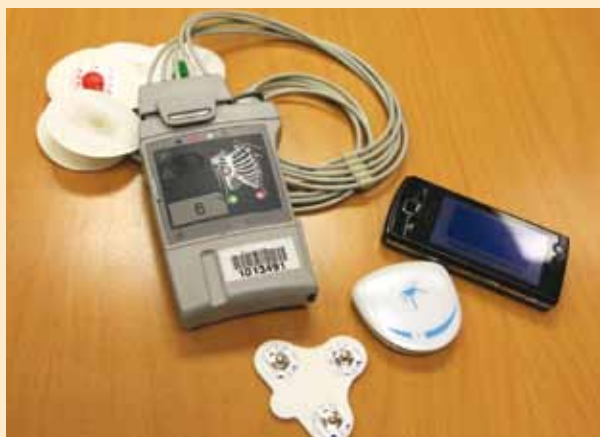
Comparison of the current holter monitoring device (top left) with the new wireless ECG monitoring system, Spyder.
