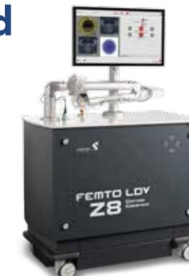
This high-speed system also allows generation of tightly focused low-energy laser pulses in an overlapped pulse raster, resulting in a complete and smooth resection for easy flap lift, and faster visual recovery.
